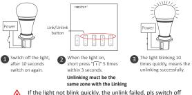
If the light not blink quickly, the unlink failed, pls switch off the light again, and follow the above steps to unlink again.
