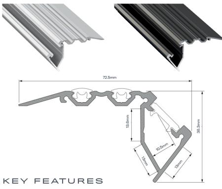
AL-STAIR is a stairs profile with built-in anti-slippery rope. Designed to be used for lighting of stairs in public spaces.
